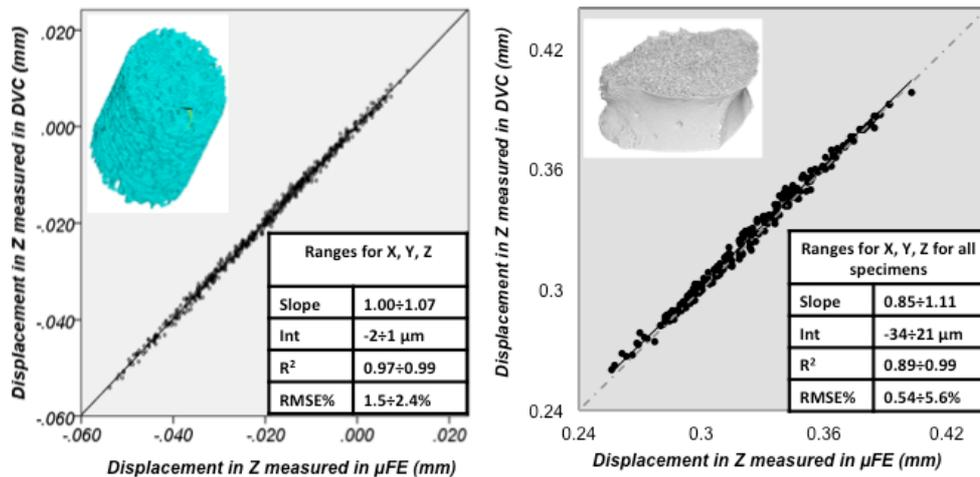
**Figure 1:** Correlation between the displacement along the loading direction measured with DVC and predicted by microFE models for the trabecular bone sample (left) and a typical vertebral body (right). In the tables ranges of the statistical parameters for every direction and every specimen are reported.
