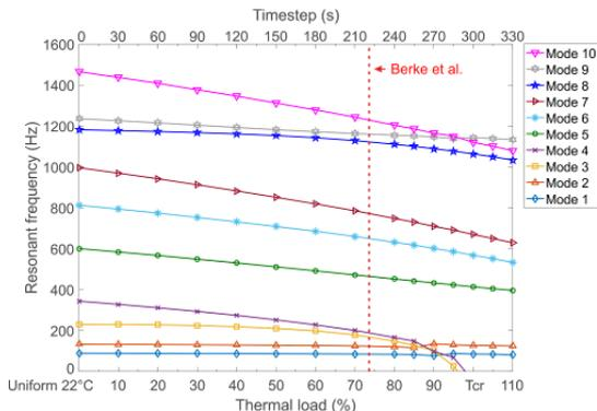
Figure 3. Resonant frequency change with  $T_{cr}$
