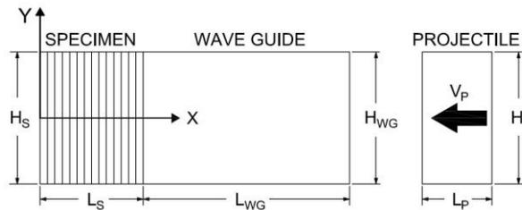
Figure 1: Schematic of simulated impact experiment. Fibres are oriented parallel to the Y axis.
