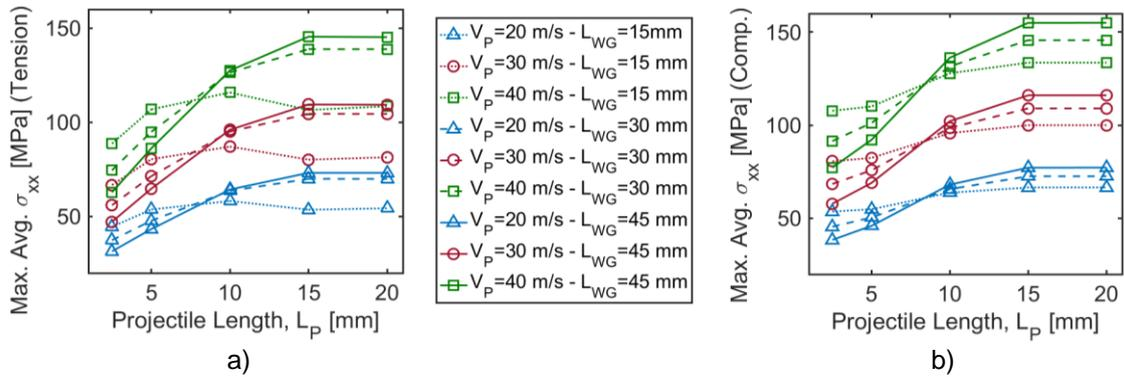
Figure 2: Simulated maximum average tensile stress (a), and compressive stress (b) as a function of varying projectile length, projectile speed and wave guide length.
