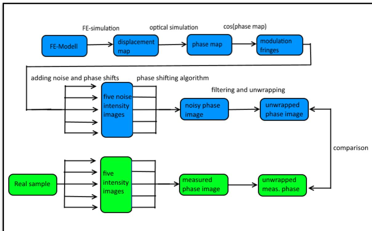
**Fig. 2** Simulation process
