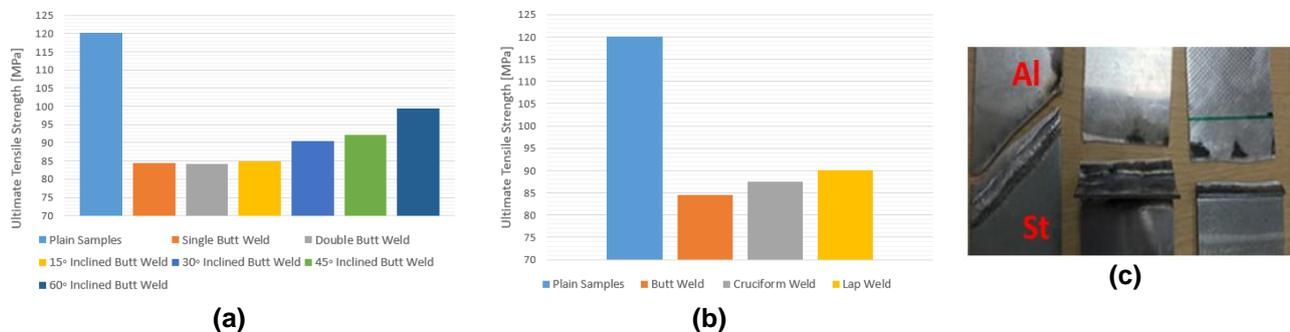
Figure 2 a) The average tensile strength results of Al-St butt, lap and cruciform Welded Joints b) The average tensile strength results of inclined angles c) tensile static failure of hybrid welded joints
