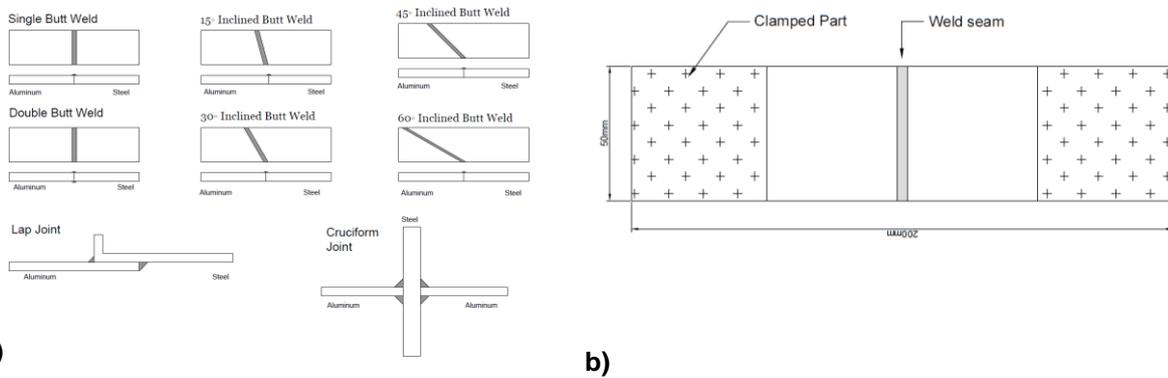
a) Figure 1 a) Geometry of investigated aluminium-to-steel welded components b) Schematisation of the tensile specimens
