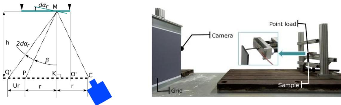
Figure 1– Principle of deflectometry (left) and typical experimental set-up [6] (right)
