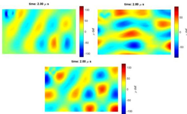
Figure 5 – Surface strains from curvatures on a glass plate with a thin patch at the back
