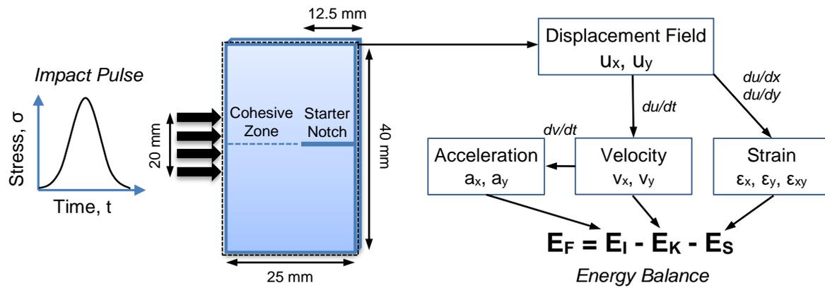
Figure 1: Schematic of proposed fracture test configuration
