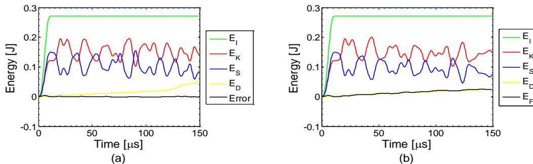
Figure 2: (a) Energy balance for the 'no crack growth case'. (b) Energy for balance for the cohesive model.
