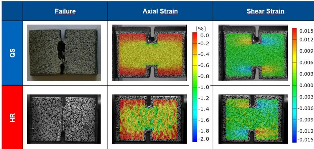
Fig. 2: Failure mode and strain fields under quasi-static (QS) and high rate (HR) loading conditions
