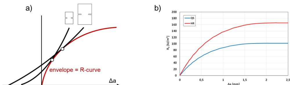
Fig. 1: Schematic illustration of the R-curve calculation methodology (a), R-curve of IM7/8552 for fiber compression failure mode at QS- and HR-loading (b)
