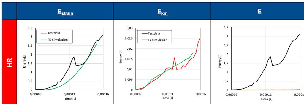
Fig. 3: Strain energy and kinetic energy curves under high rate loading, based on DIC and FE-simulation
