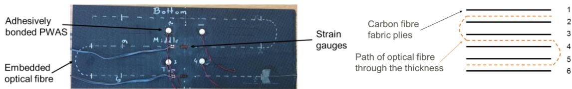
Figure 1. Network of sensors in finished panel (left) and integration of OFS through-the-thickness of the panel (right)
