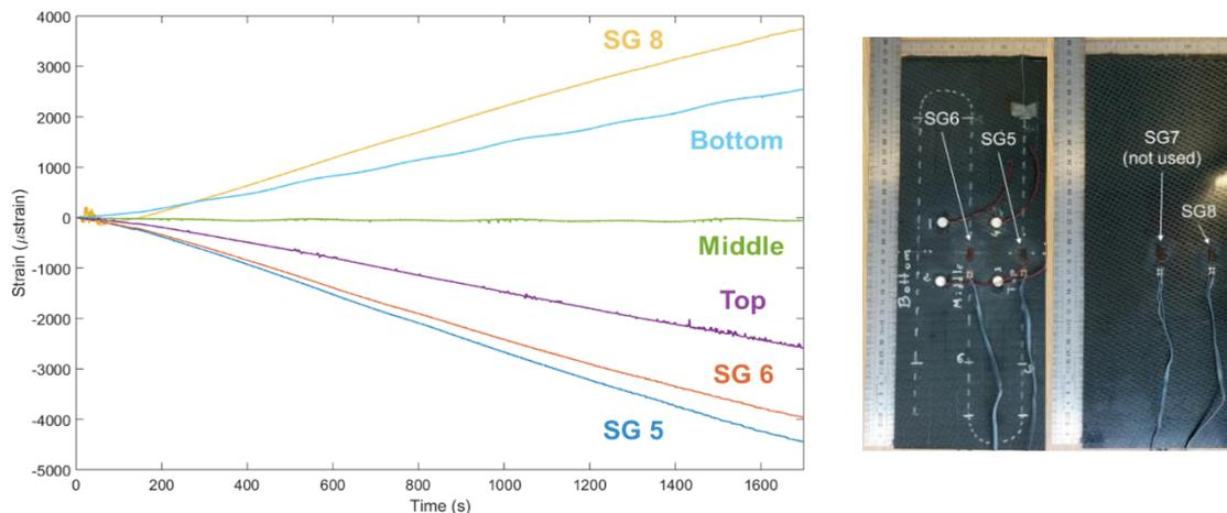
Figure 3. Comparison of strain recorded by strain gauges and OFS during fifth loading
