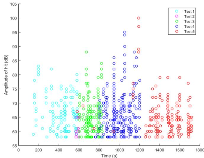
Figure 2. Amplitudes of AE hits recorded during the first five loadings
