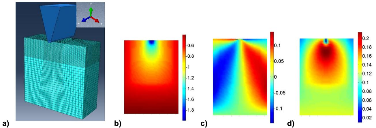
Figure 1: a) Finite element model of a rubber block (60mmx60mmx25mm) subject to a 2mm indentation by a rigid wedge and the corresponding displacement maps in b) X, c) Y and d) Z directions.
