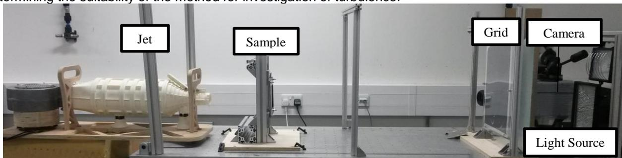
Figure 1: Experimental setup
