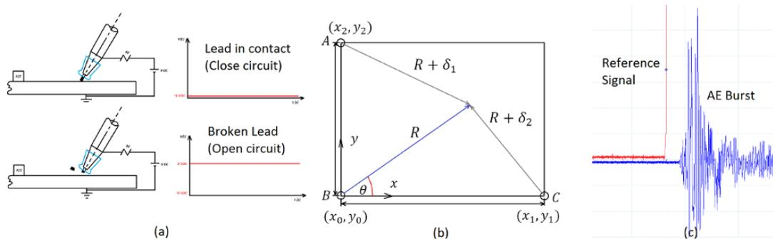
Fig 1: (a) Triggering mechanism, (b) Triangulation of an AE source and (c) Reference signal
