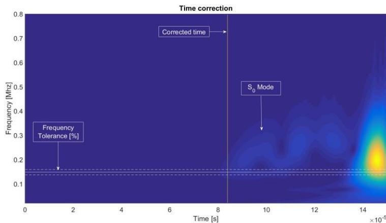
Fig 2: CWT of an AE burst
