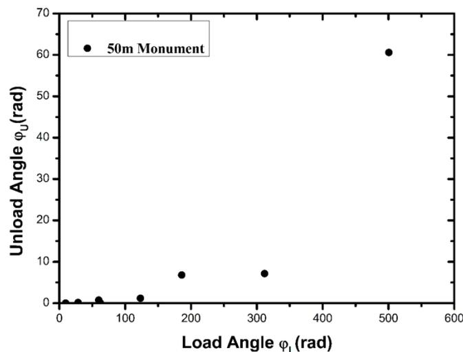
**Fig.5:** Preliminary data for the 150 $\mu$ m copper wire, gauge length 50m.
