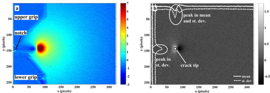
**Fig. 1. a) Results of post-processing on one TSA image: a) Normalised magnitude b) Difference image comparing normalised image with that of previous time step, showing crack tip position found by the algorithm and the mean and standard deviation of each row and column of pixels.**
