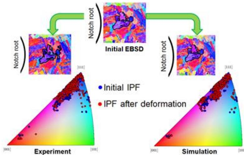
Figure 2: Experimental and simulated change in inverse pole figures (IPF) after deformation at 500C
