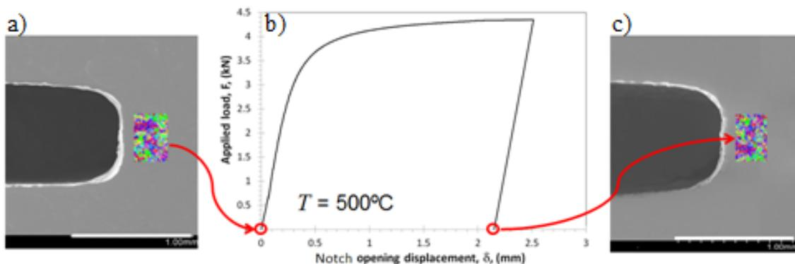
Fig 1: Experimental procedure: a) Position of the initial EBSD scan, b) Force vs notch opening displacement responds at 500C, c) position of the EBSD scan taken after unloading
