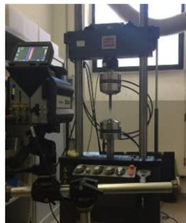
Figure1: Experimental set-up adopted for thermographic tests.
