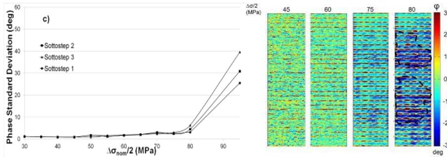
Figure 2: Sample 3: (a) Phase Standard Deviation parameter in three sub-steps, (b) phase maps.
