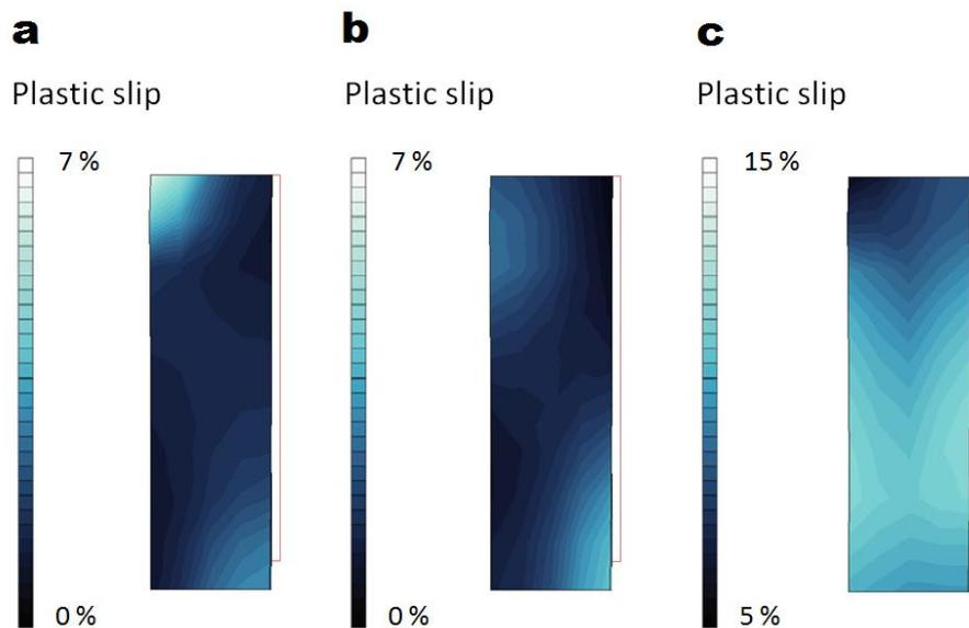
**Figure 2:** A typical example of the type of crystal plasticity results that have been obtained to enable a one-to-one comparison with the micro-tensile experiments: Plastic slip activity one of the constrained specimens, e.g. G1S3 or G1S4. (a) Activity of the  $(110)[111]$  slip system; b. Activity of the  $(110)[111]$  slip system; and c. Activity of the  $(120)[111]$  slip system.
