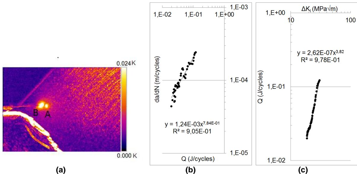
Figure 2 results (a) map of the amplitude  $T_2$  (b) relation between  $da/dN$  and energy dissipated  $Q$  (c) relation between energy dissipated  $Q$  and  $\Delta K_I$ .
