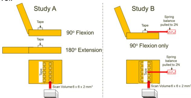
Fig. 1: Loading arrangements for studies A and B. Original setup detailed in Maiti et al. [3].
