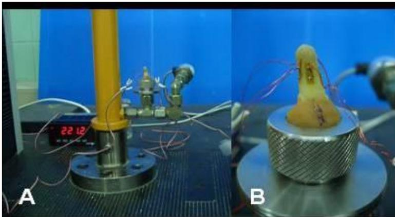
Fig. 1: (A) Experimental setup (B) Close-up of the tooth root with the strain gages
