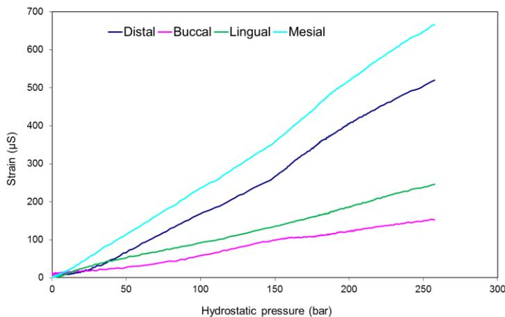
Fig. 3: Strains – pressure diagrams obtained during loading a maxillary incisor.
