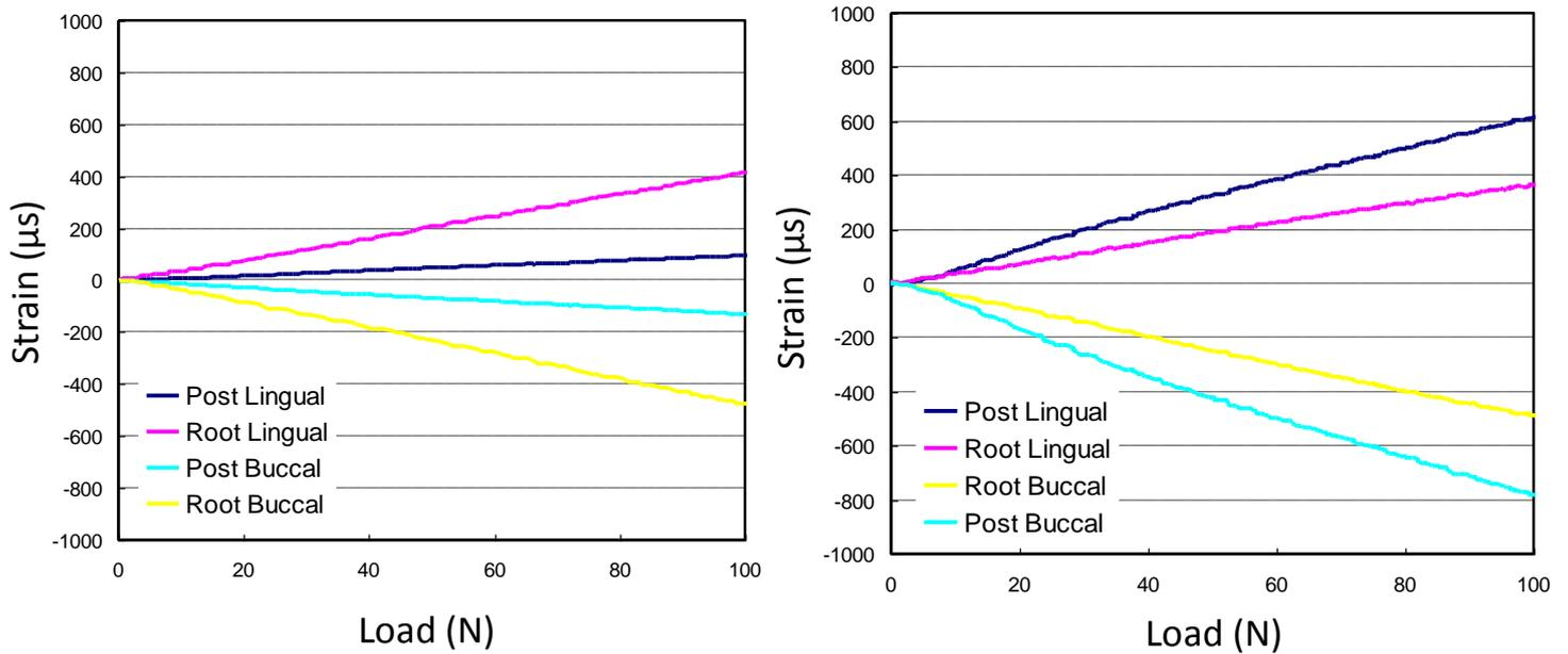
Fig. 1 Strains on post and root at 5mm ferrule (left) and 0mm ferrule (right) while loading the cemented crown at 30°. Note that the strains on the root were similar whereas those on the post increased >6 fold.
