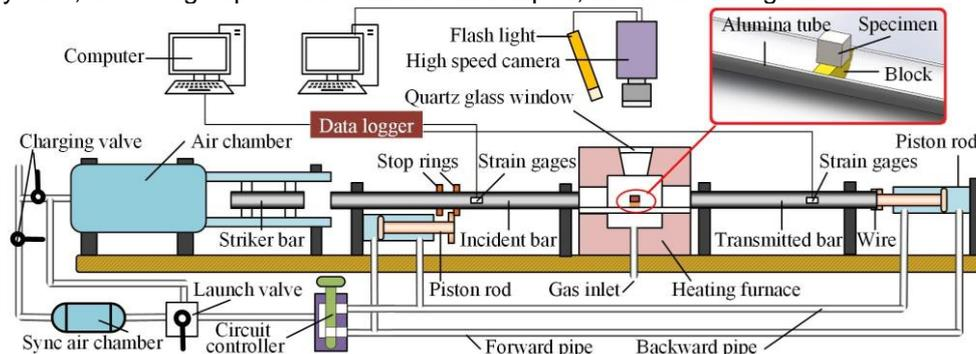
Fig. 1 Schematic illustration of the high temperature split Hopkinson pressure bar with a double-synchronous assembled heating system and a high speed camera.
