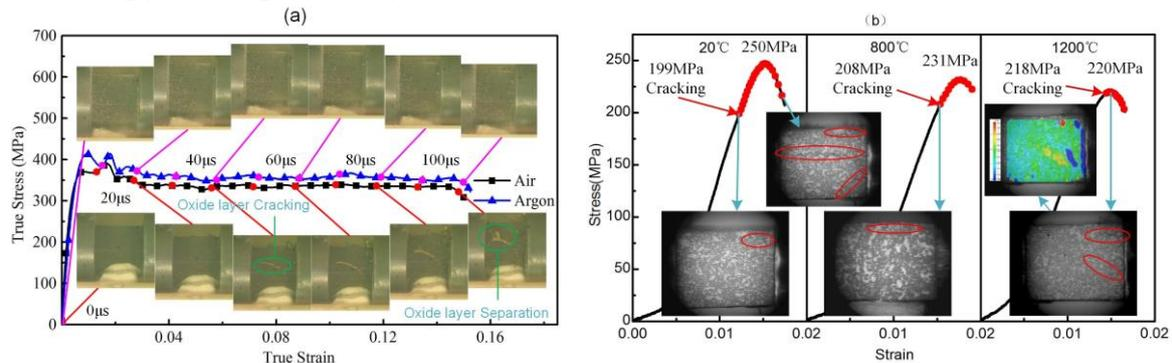
Fig. 2 (a) Stress-strain curves and image at 2000 1/s and 1100 C in different environments; (b) true stress vs. true strain at different temperatures (at the rate of 200 1/s)
