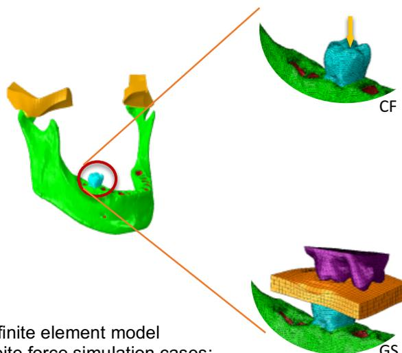
Figure 2: Jaw finite element model including two bite force simulation cases: concentrated point force (CF), and gold standard bite force distribution at the occlusal surface (GS)
