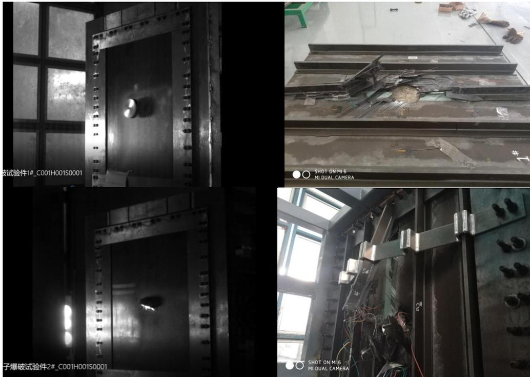
Fig. 2 High speed photos and visible damage for composites impacted by projectiles with different attitude
