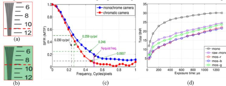
Fig. 3 Evaluation results for monochromatic and chromatic images. (a)/(b) spatial resolution of monochromatic/chromatic images, (c) /(d) MTF/SNR of monochromatic and chromatic images.
