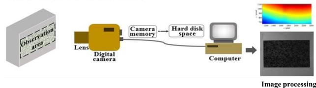
Fig.1 Main procedures for photomechanical measurement.
