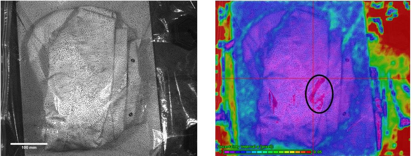
Fig. 1: Left, camera one image from Vic-Snap 8, of a lab coat placed within speckled vacuum bag. Right, the uncertainty estimate produced by Vic-Snap 8, for a step size of 61 pixels. The region highlighted with a black circle shows there is some oversaturation, caused by high reflectivity of the bag, to be taken into account.
