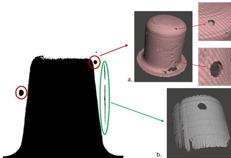
Fig. 2 Defects observations within the cement layer. a) voids, b) partial debonding
