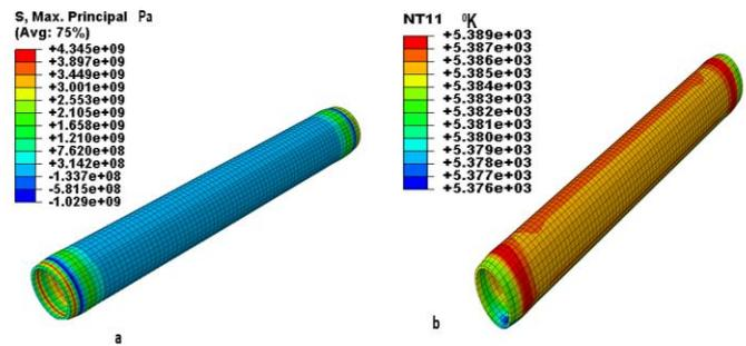
Figure 2 (a) Max principal stress (MPa), (b) Nodal temperature (K)
