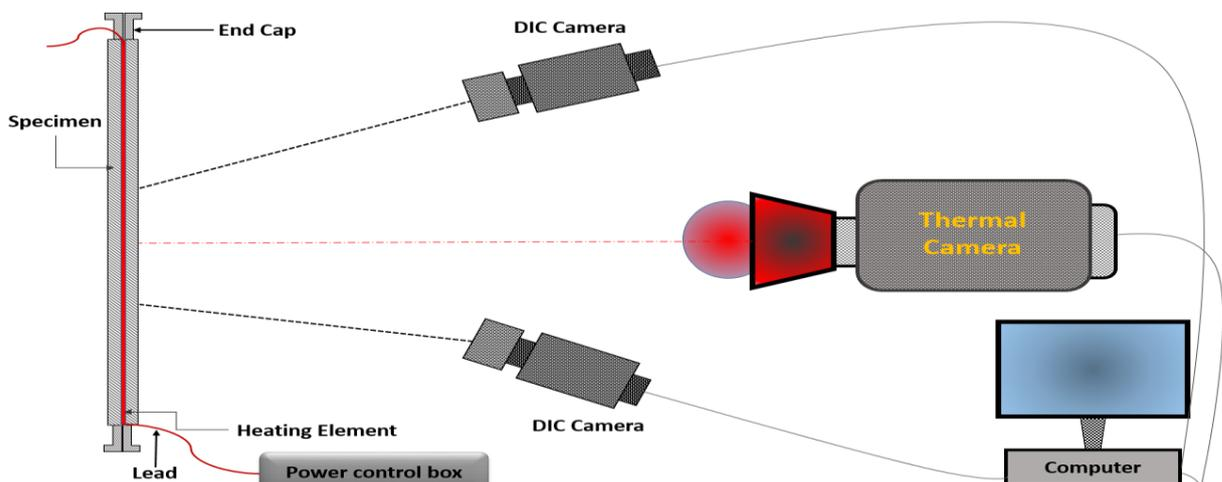
Figure 1 DIC experimental setup for full-field thermal analysis
