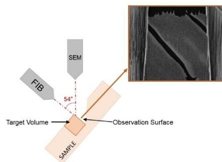
Figure 1 : Scheme of FIB-SEM "Slice and View" principle.
