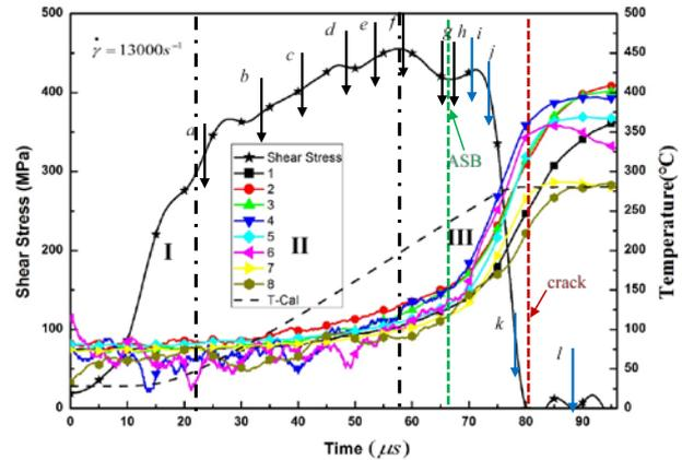
Fig.2. Deformation process of a shear-compression test. The arrows *a~i* indicate the time of camera shot, as shown in Fig.3. 1~8 represent the elements of IR measurement. T-Cal is the calculated temperature based on the conversion of mechanical work to heat (taking 1.0 as Taylor-Quinney factor). The dashed green line and red line denote the appearances of ASB and crack, respectively.
