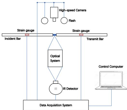
Fig.1. Arrangement of the SHPB apparatus combined with high-speed photography and temperature measurement system
