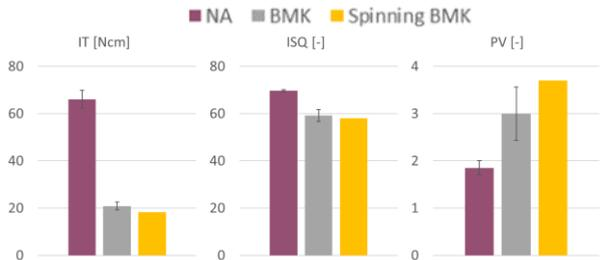
Figure 2 Anchorage measurements (IT, ISQ, PV) at implant insertion (prior to loading). Mean  $\pm$  standard deviation
