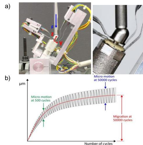
Figure 1 Dynamic loading test setup. a) Sensor system with unit positioning; b) Visualization of Migration (Mig) and micro-motion (MM)
