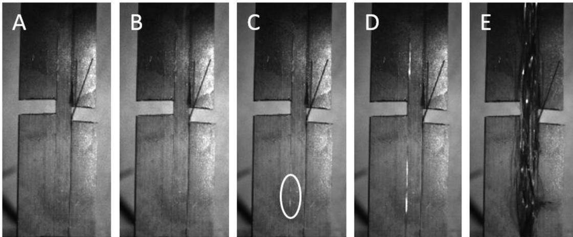
**Fig. 1 Failure of a unidirectional carbon-fibre laminate in tension. Kirana triggered autonomously via acoustic system (500,000 fps). (A) 2  $\mu$ s before trigger. No evidence of premature triggering. (B) 0  $\mu$ s after trigger. (C) 2  $\mu$ s after trigger. First evidence of fibre failure (highlighted area). (D) 12  $\mu$ s after trigger. (E) 192  $\mu$ s after trigger.**
