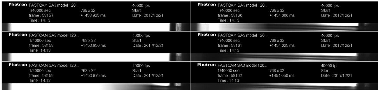
Figure 2: High-speed, curved-fronted, discrete liquid jet produced by experimental equipment
