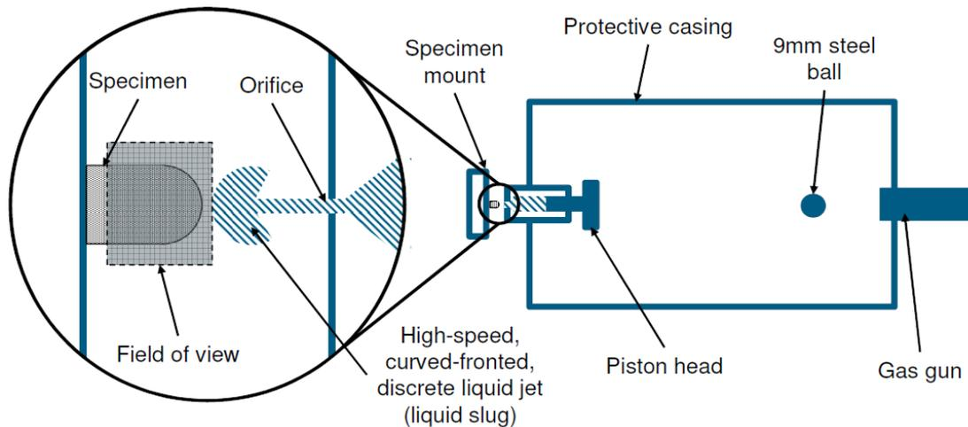
Figure 1: Experimental set-up for producing high-speed droplet impingement on specimen with grid pattern.
