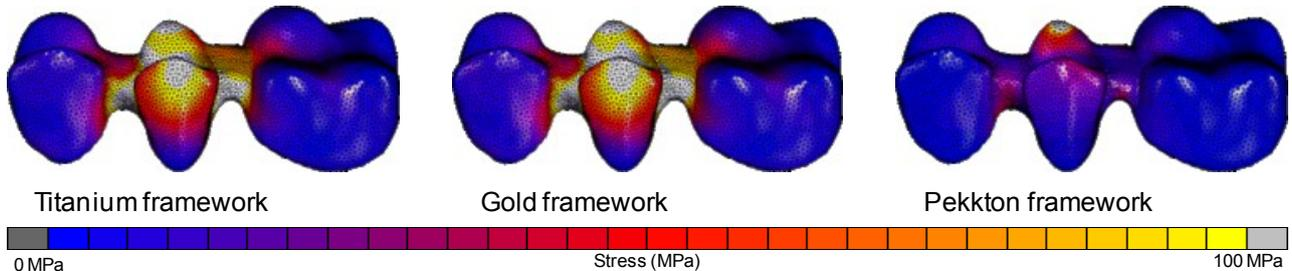
Fig. 2: Computed stresses in the framework of the three-unit bridges for a load of 500 N depending on the framework material.
