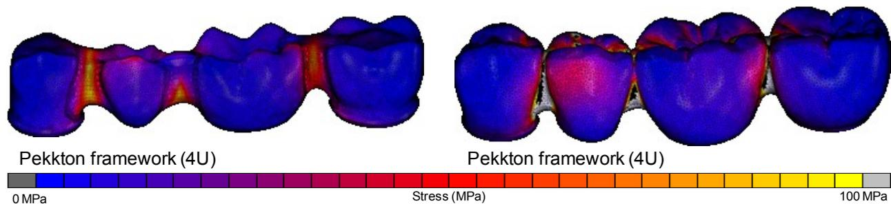
Fig. 4: Computed stresses in the framework (left) and the veneering (right) of the four-unit bridges with polymer framework for a load of 500 N.
