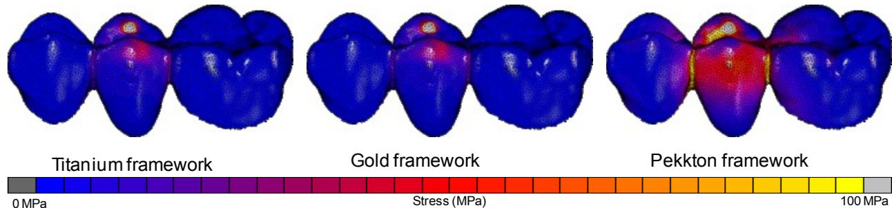
Fig. 3: Stresses in the veneering of the three-unit bridges for a load of 500 N depending on the framework material.
