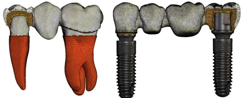
Fig. 1: FE models of the three-unit (left) and four-unit bridge (right). Part of the model is cut away to show the inner composition of cement, framework and veneering.
