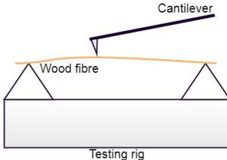
Figure 1: The testing schematic for the three-point-bend testing of wood fibers using AFM. A stainless steel rig, with two knife edges two millimeters apart, supports a single wood fibre. After measuring the dimensions of the fibers, the AFM engages with the centre of the fibre: the load is applied here and the resulting displacement measured.
