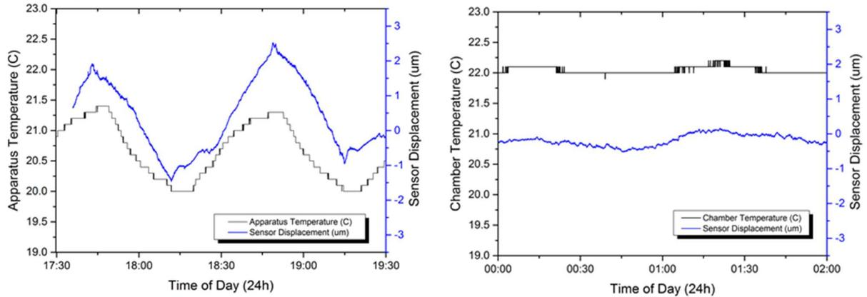
Figure 1 - Graphs of apparatus ambient temperature and the sensor displacement without apparatus enclosure (a) and with apparatus enclosure (b), indicating a relationship between sensor displacement and apparatus ambient temperature. The use of a thermal enclosure leads to a significant reduction in chamber and apparatus temperature variation which in turn minimises sensor displacement, resulting in a more stable scanning outcome.
