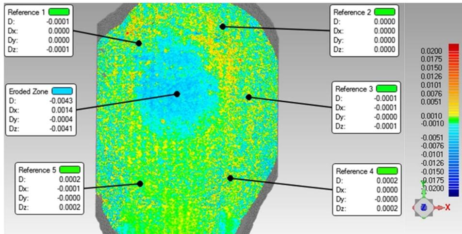
Figure 2 - Representative example of a sample with its associated wear scar in blue, green denotes no change, whilst yellow denotes gain post erosion. Wear scar depth is depicted by 3D total deviation (D) and Z-deviation (Dz). The central eroded region and 5 reference regions have been analysed for allow for erosion versus non-eroded comparison. This indicates a wear scar depth of 4.3  $\mu\text{m}$ .
