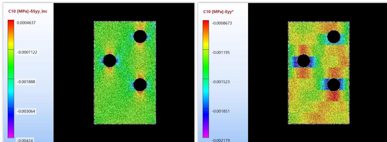
Figure 1: Incremental stress sensitivity map for C10 at 0.5 N (left panel) and corresponding longitudinal virtual strain field adopting a 9x9 virtual mesh.
