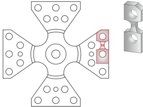
Figure 1 – Hour-glass specimen geometry.
