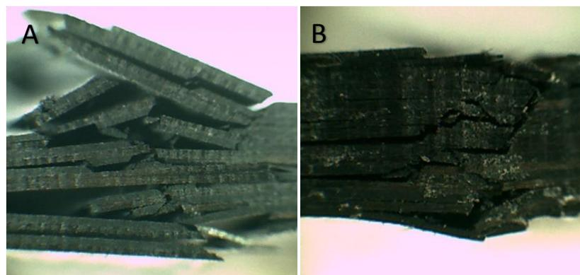
Figure 2: Failure modes obtained for UD specimens after the compression test: A is wet and B is dry.
