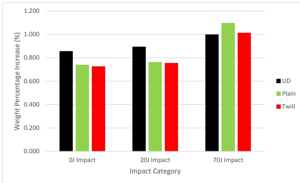
Figure 1: Water uptake for undamaged, after 20 joules impact damage, and after 70 joules impact damage for CFRP specimens.
