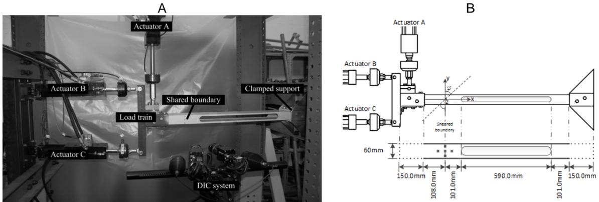
Figure 2: Test rig: a) overall test setup including load train, DIC system, etc. and b) overall dimensions
