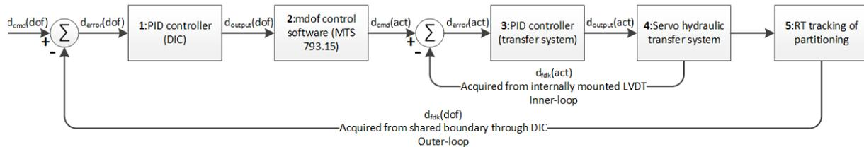
Figure 1: schematic block diagram representing the cascade control loop algorithm
