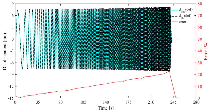
Figure 3: compensator performance with a chirped sine wave in the domain 0-2Hz
