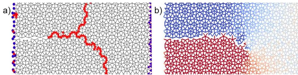
Figure 2: Lattice simulations. a) crack path and b) iso-contour of the rotation field
