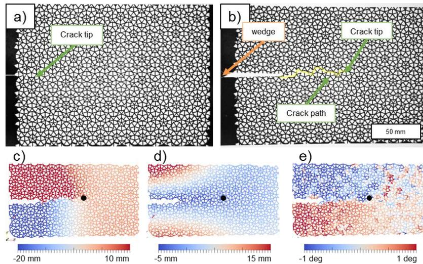
Figure 1: Fracture tests on Penrose tiling-based PMMA specimens. (a) Image at rest, (b) loaded state, (c) and (d) the measured transverse and axial displacement fields and (e) the rotation field.
