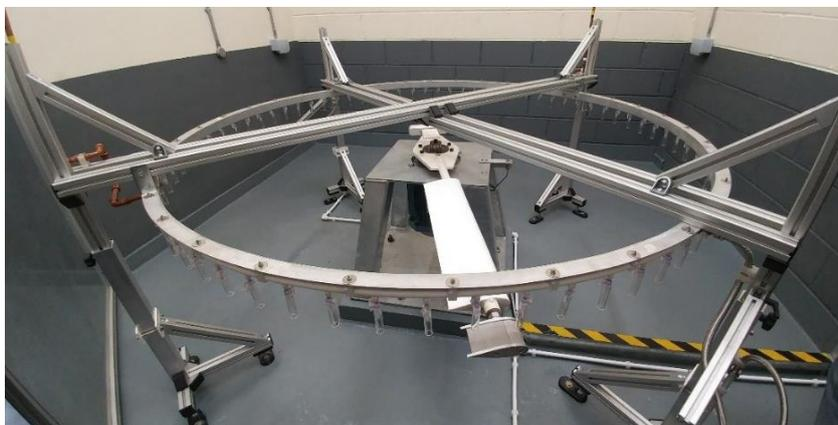
Figure 1- Setup of ETC's Erosion Test Rig
