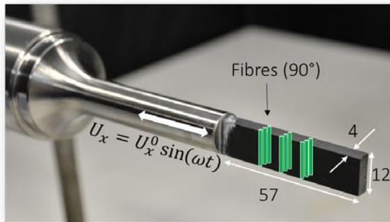
Figure 1: Ultrasonic testing configuration
