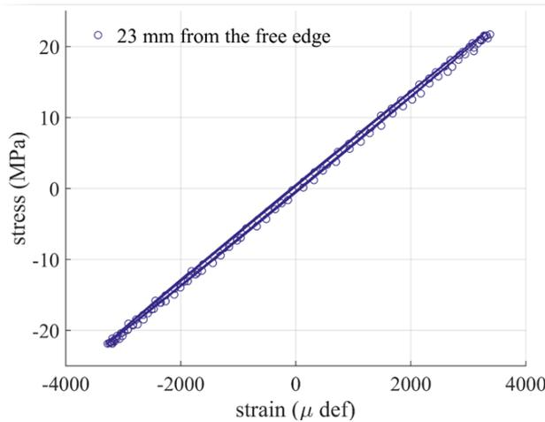
Figure 3: Stress-strain curve just before fracture
