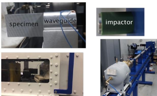
Figure 1: Direct inertial impact - specimen and waveguide, impactor, impact chamber with specimen and gas gun (left to right, top to bottom)
