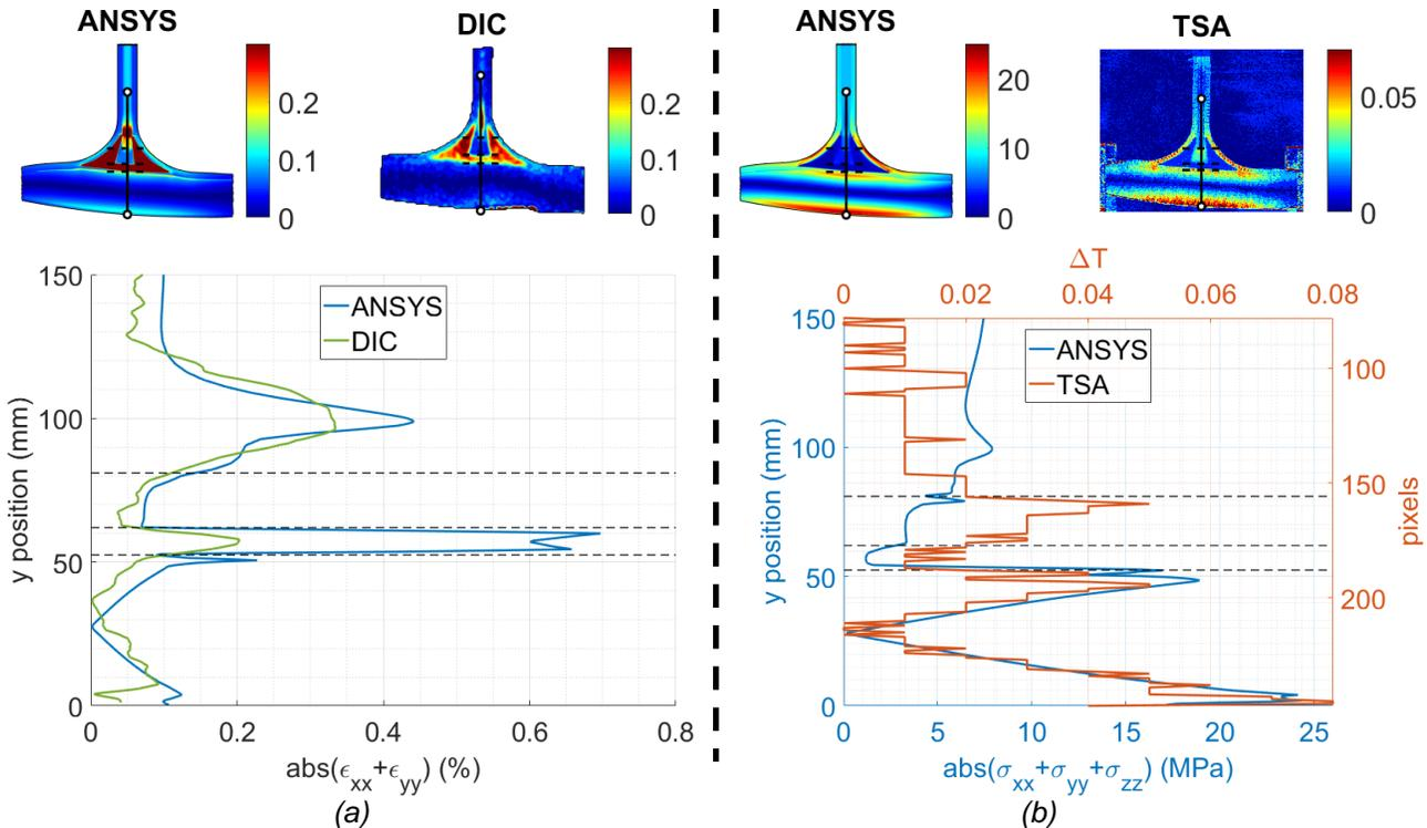
**Figure 2:** Numerical and experimental result comparison by surface contours and midline plots – (a) sum of surface in-plane normal strains from FE and DIC; (b) sum of surface normal stresses from FE and change in temperature from TSA
