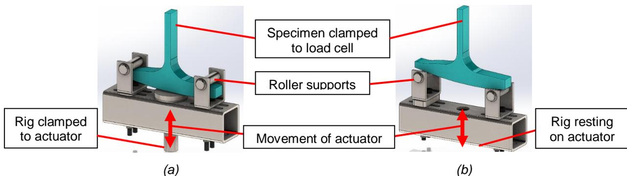
**Figure 1:** 3PB load rig configurations – (a) Tension; (b) Compression
