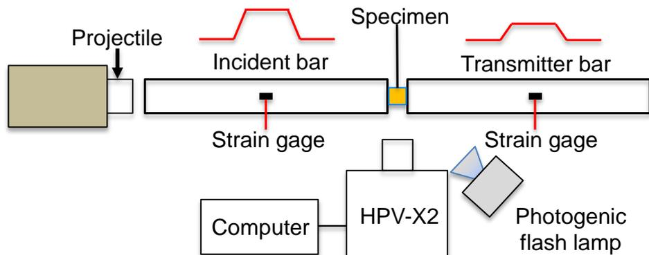
Fig . Experimental Setp up (Hopkinson bar with high speed imaging)
