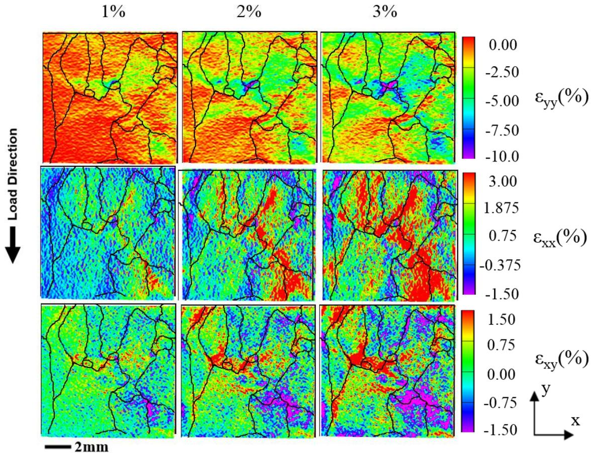
Fig.2. Typical local full field strain in pure magnesium
