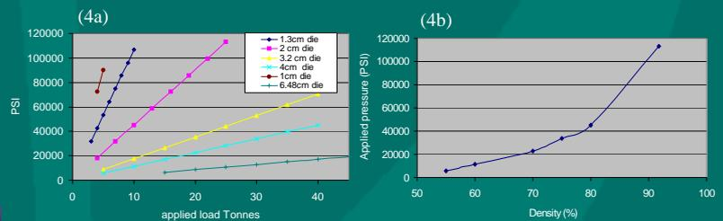
Figure: 4 a) Actual pressure as a function of applied force for different diameter dies and b) Density as a function of pressure for the copper particles.
