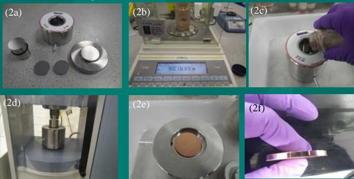
Figures: 2 a) Die assembly for pressing copper disc 2b) Weighing out powder required 2c) pouring of powder in die 2d) die in press ready for pressing 2e) Copper powder after pressing in the die 2f) disc removed from die.
