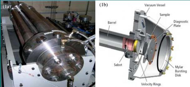
Figure 1: a) AWE Helium Gas gun and b) Target chamber.
