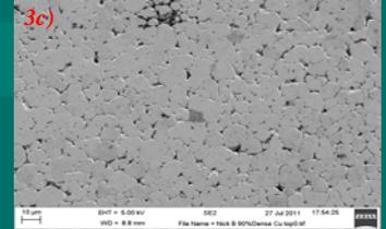
Figure 3: SEM image for the copper powder in a) its free form, b) after pressing into a 63% dense disk and c) a 90% disk.
