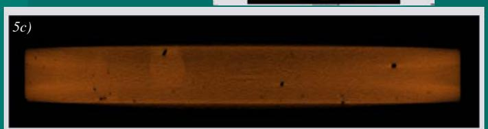
Figures: 5 a-c) X-ray tomography of pressed copper disks
