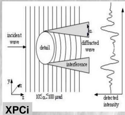
The physical quantity causing a phase shift can be up to 1000 times larger than the one responsible for attenuation.
