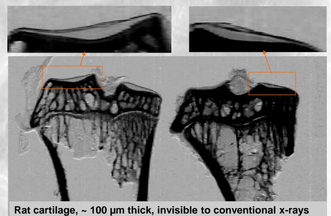
Rat cartilage, ~ 100 μm thick, invisible to conventional x-rays
