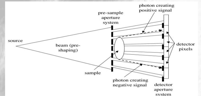
The use of coded apertures makes XPCi feasible in the lab
