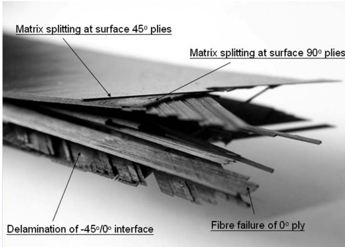
Multiple failure mechanisms that may interact
