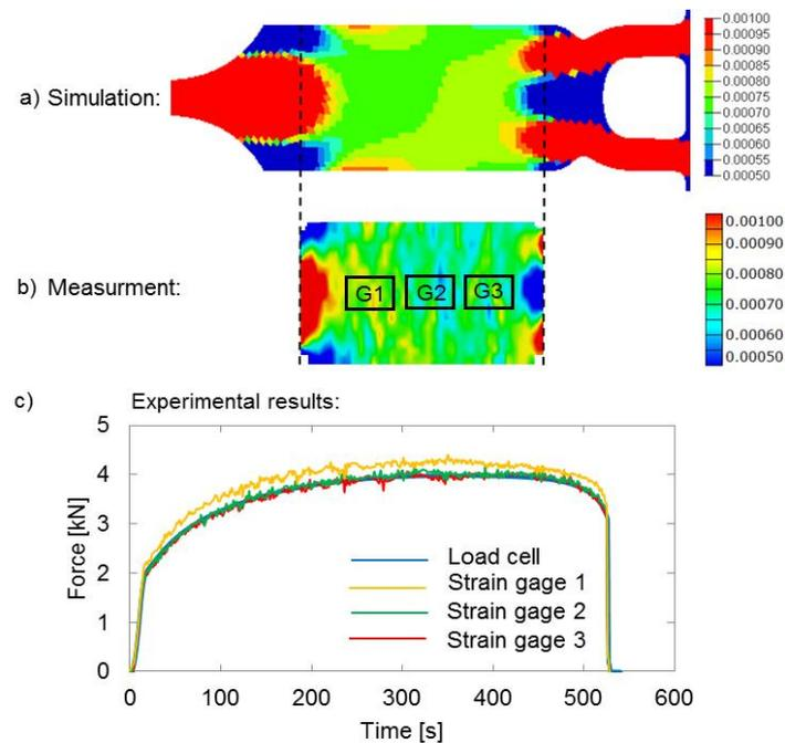
Figure 2: Special geometry for a homogeneous elastic strain field
