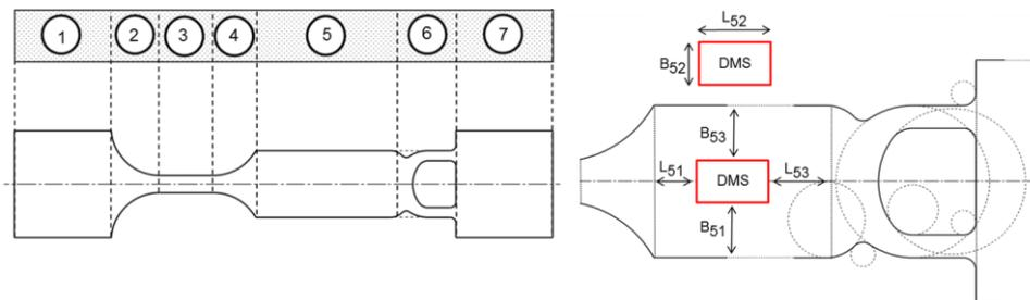
Figure 1: A new sample geometry for ringing-free force measurement in DMS-area
