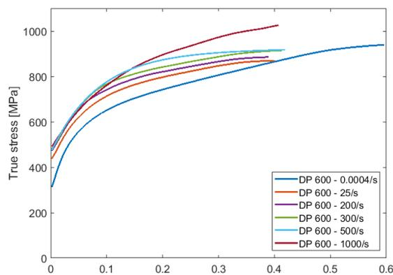
Figure 3: Example stress-strain curves of a dual phase steel DP 600
